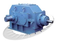
**SHAFTS** - Output shafts are made of heat treated, Maximum strength carbon steel, through hardened prior to turning and grinding. Close tolerance bearing shoulders facilitate the mounting of bearings. Highly polished surfaces are provided for oil seals to assure their long life. Large diameters are specified throughout for maximum strength and overhung load capacity.
